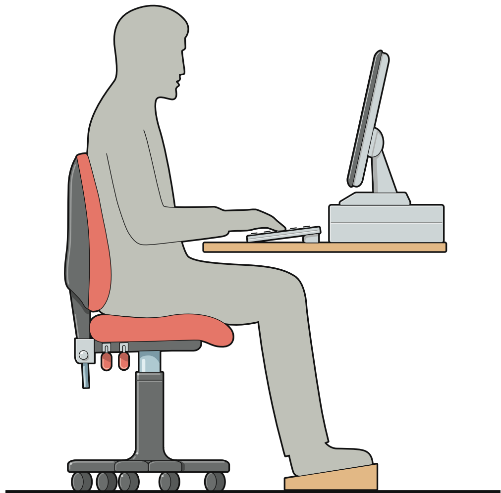
Figure 2 Seating and posture for typical office tasks
